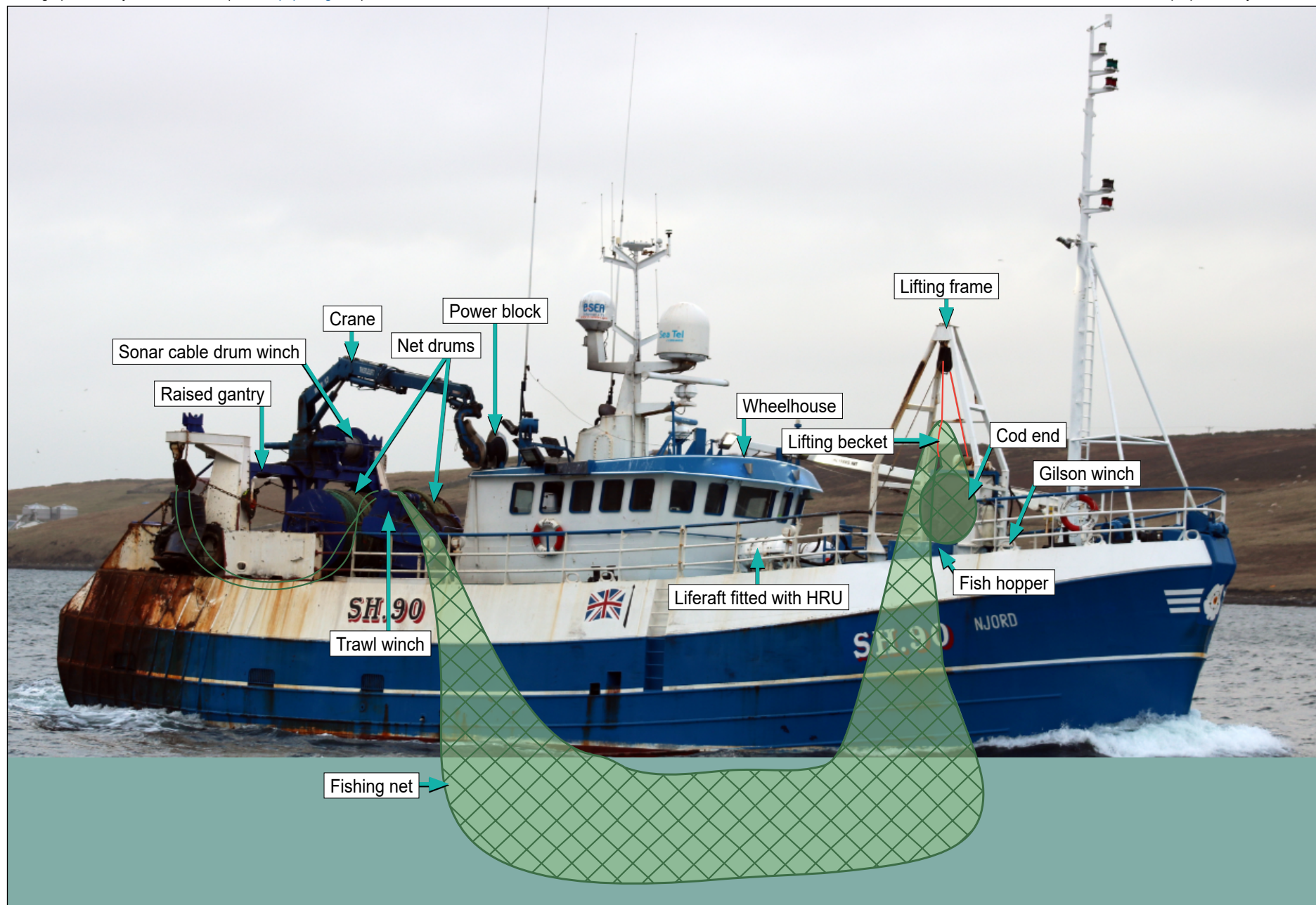
Figure 2: Njord net indicative lashing and general layout
