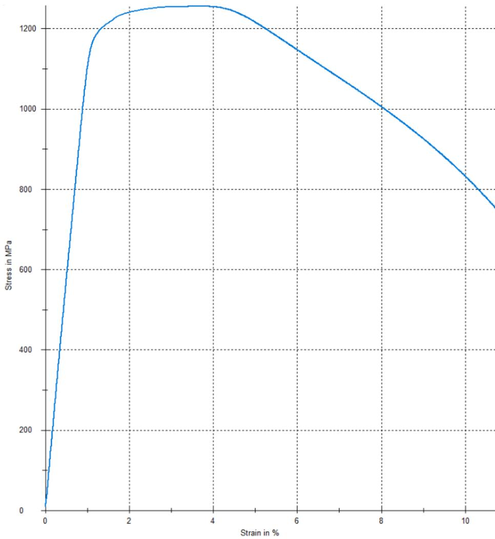
Figure 3-11 Sample MJA/4, stress-strain plot from tensile testing.
