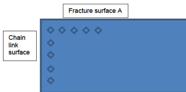
**Figure 4-42 Position of the hardness measurements on the cross section through the fracture initiation area (fracture surface A). The indents are positioned 1 mm from the chain link surface/fracture surface and 1 mm from each other.**
