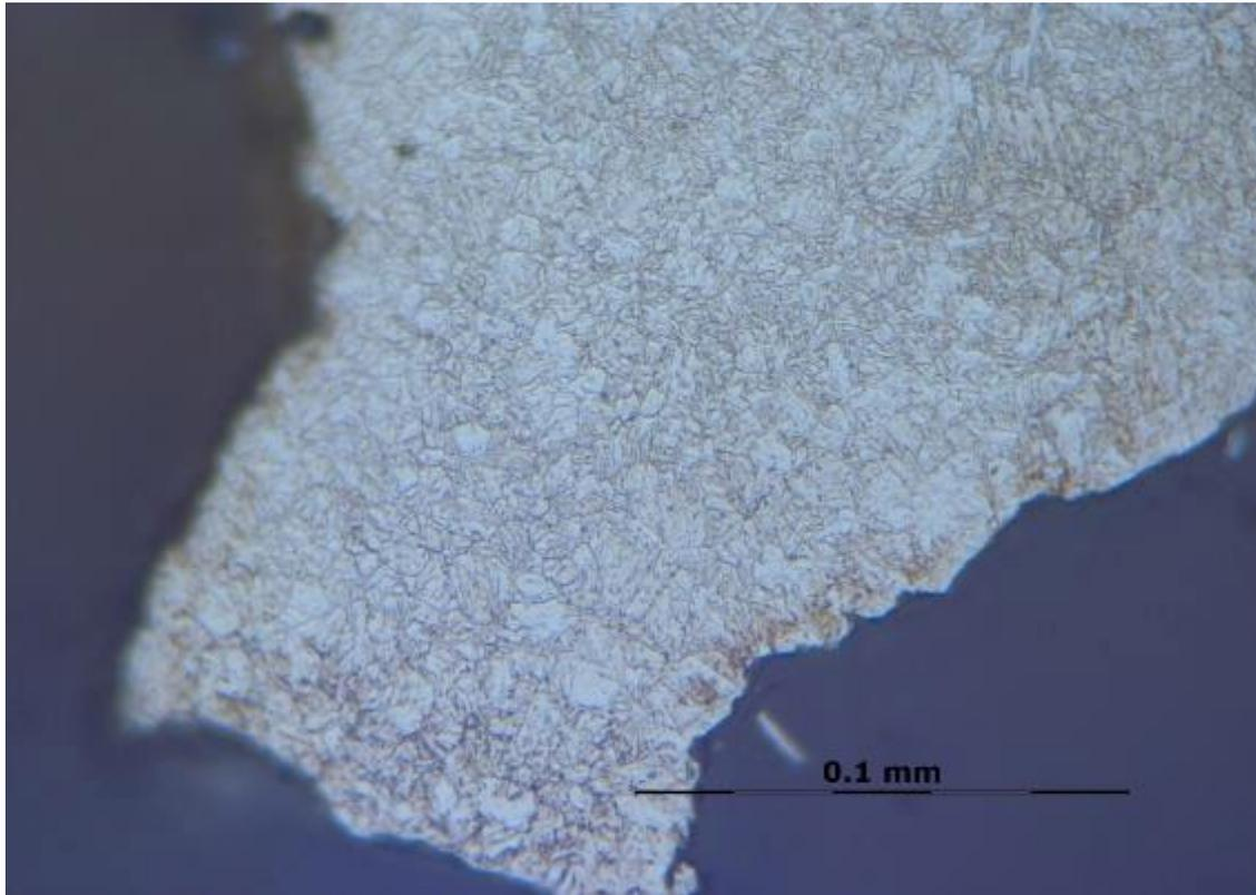
**Figure B-8-1** Cross section, link BJC/1-5: Quenched and tempered microstructure close to outer surface.
