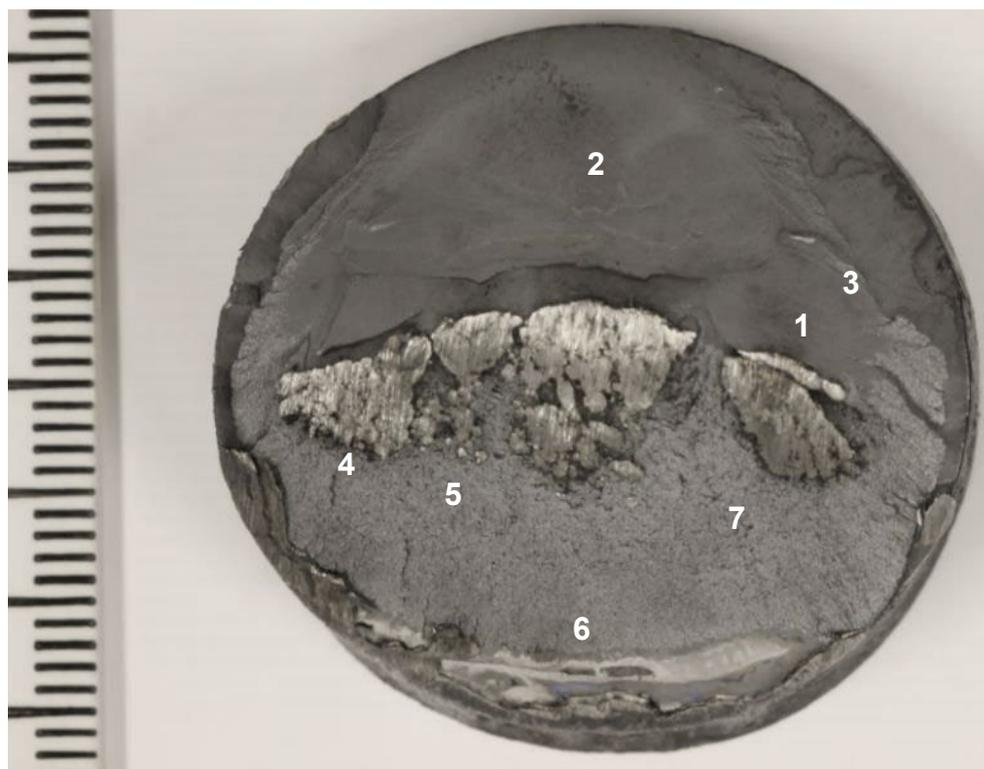
**Figure 3-23 Part MJA/4: Overview image showing the approximate position of SEM images.**
