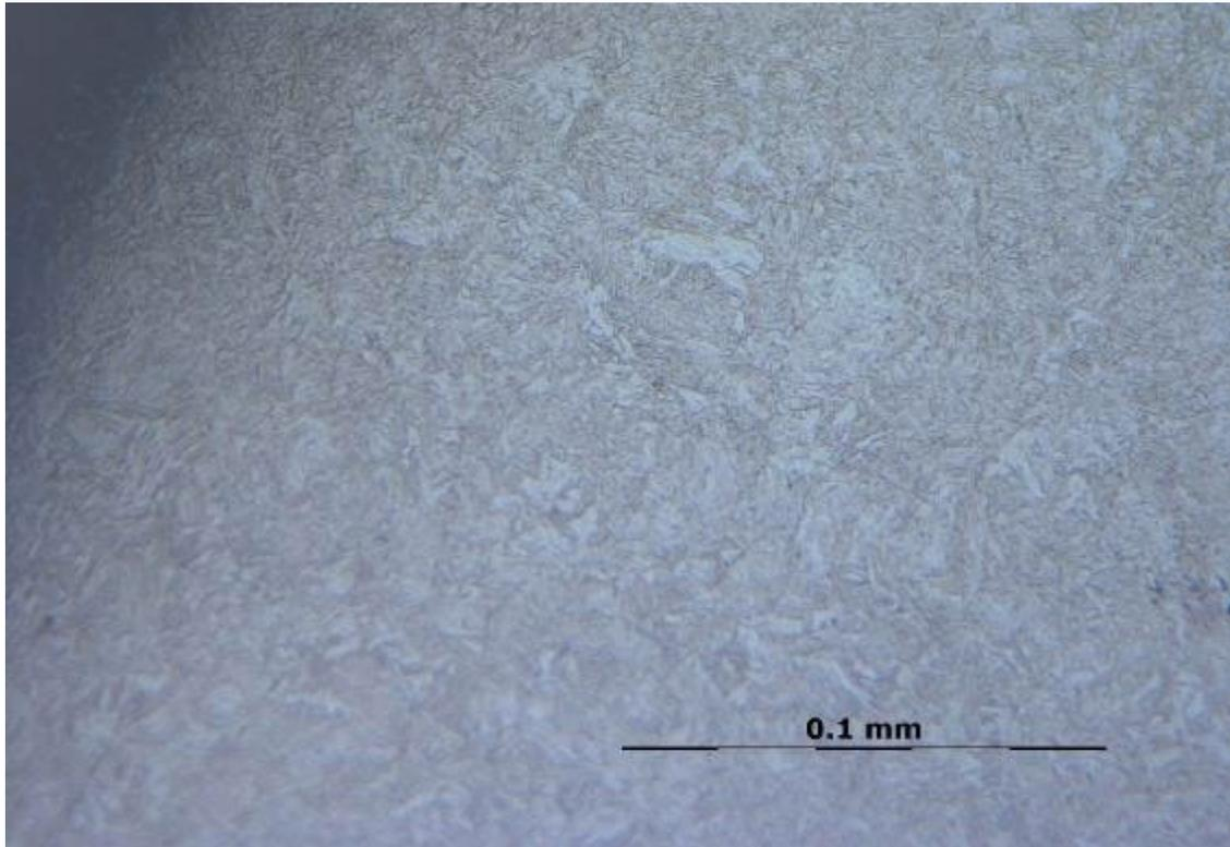
**Figure B-8-3** Cross section, link BJC/2-9: Quenched and tempered microstructure close to outer surface.
