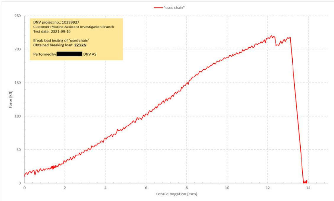
Figure 4-45 Part BJC/3, starboard used chain, tension versus total elongation.
