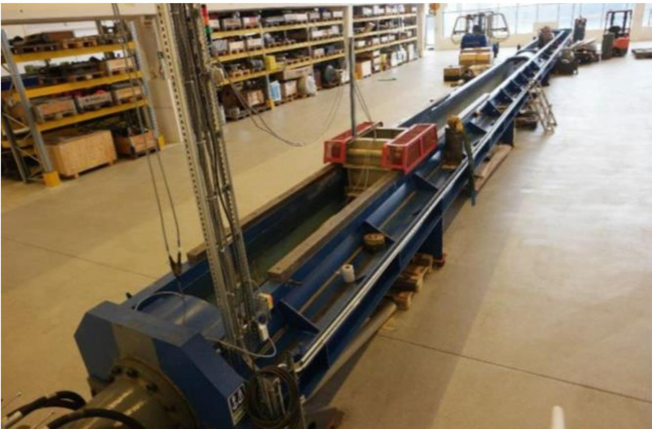
**Figure 3-15** 3,200 kN tensile capacity (designated "Ormen Lange") test machine. Note that the machine has been relocated after the image was taken.
