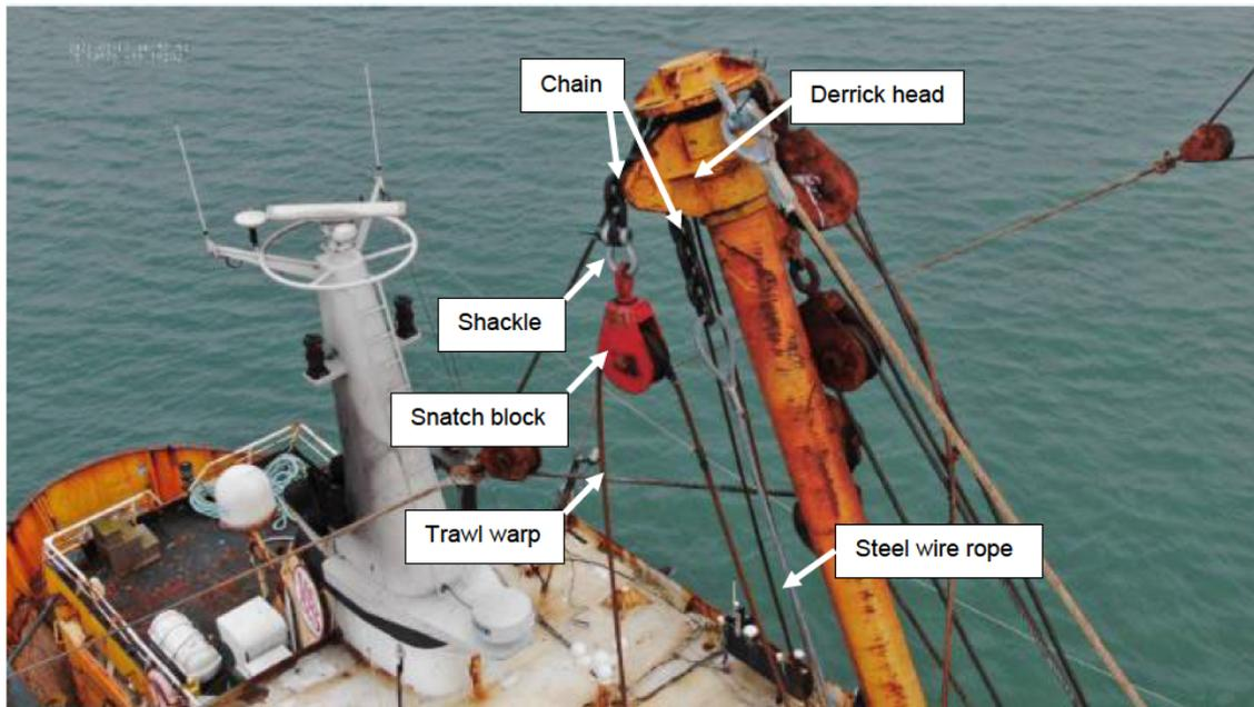
**Figure 2-1** Examples of quick release system similar to the one that failed. Image supplied by the client.
