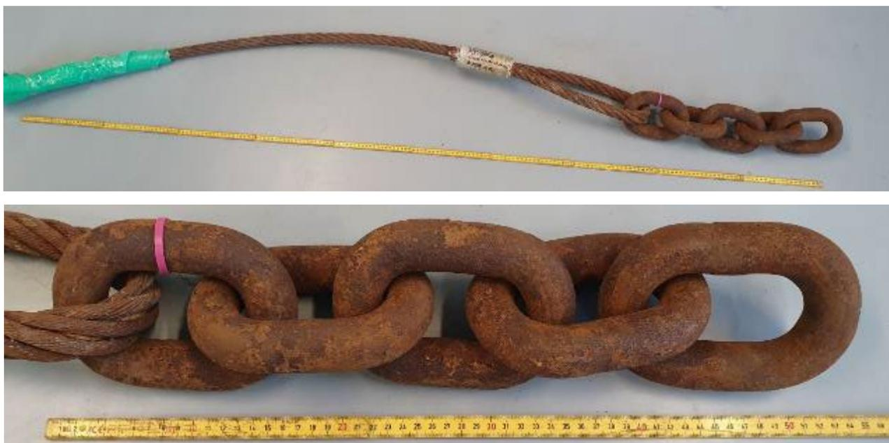
Figure 4-1 Sample BJC/1, part of portside chain, connected to steel wire rope. The upper image shows both chain and steel wire rope part, the lower image shows the chain at higher magnification.
