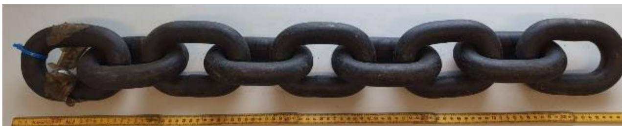
Figure 4-2 Sample BJC/2, unused (reference) section of chain.
