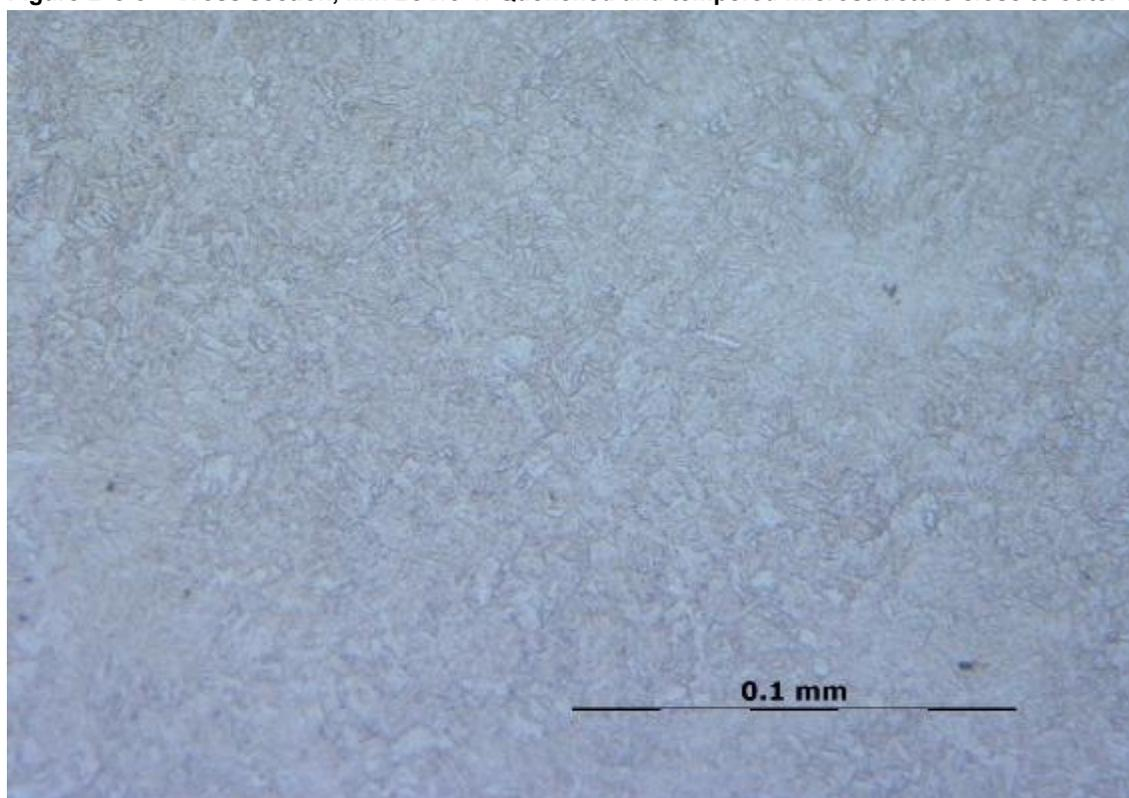
**Figure B-8-6** Cross section, link BJC/3-1: Quenched and tempered microstructure ca 10 mm from outer surface.
