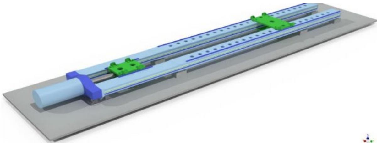
**Figure 4-43** Illustration of 28.5 MN capacity tensile tester's test bed.
