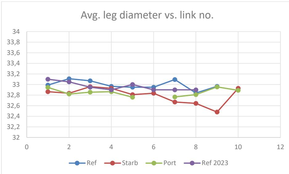
**Figure 3-9** Measured average leg diameter plotted versus link number for all examined chain segments.
