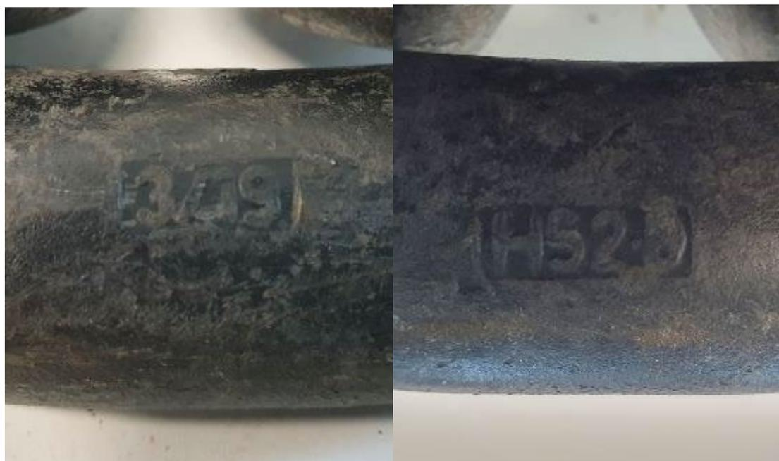
**Figure 4-16** BJC/2 –Marking on unused chain link.
