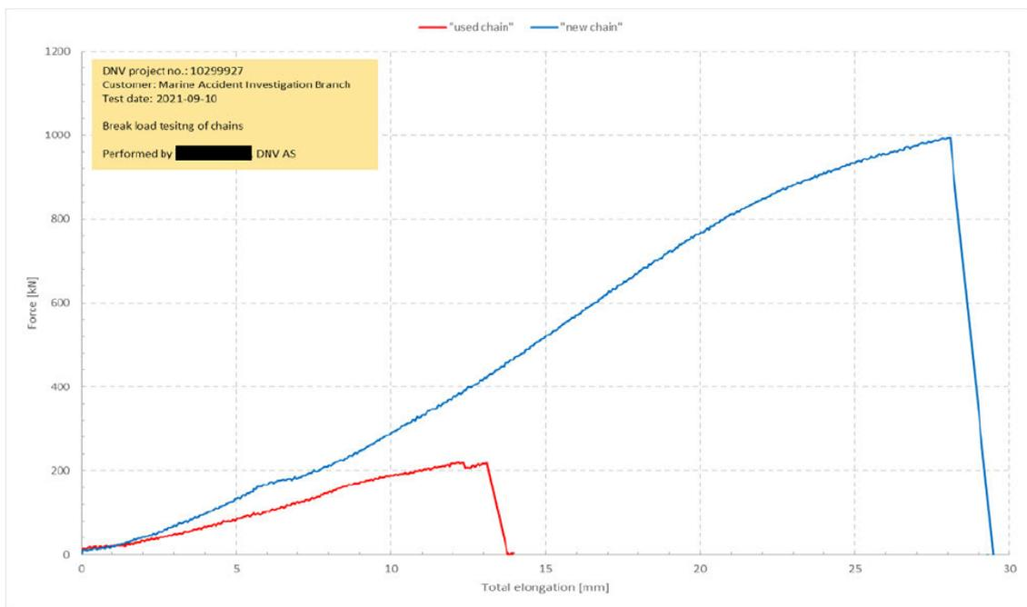
Figure 4-46 Part BJC/2, unused reference chain (blue) and Part BJC/3, starboard used chain (red), tension versus total elongation.
