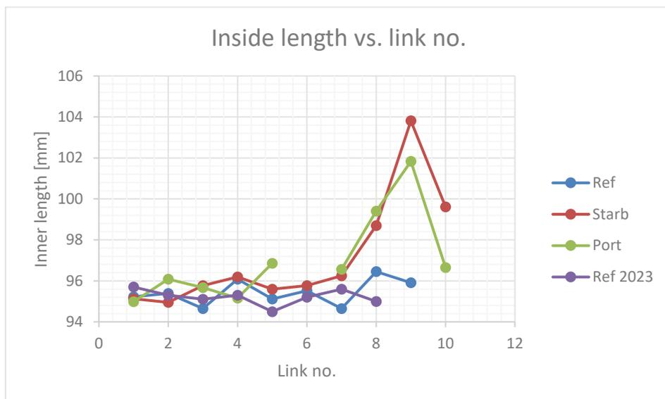
**Figure 3-7** Measured inner length plotted versus link number for all examined chain segments.
