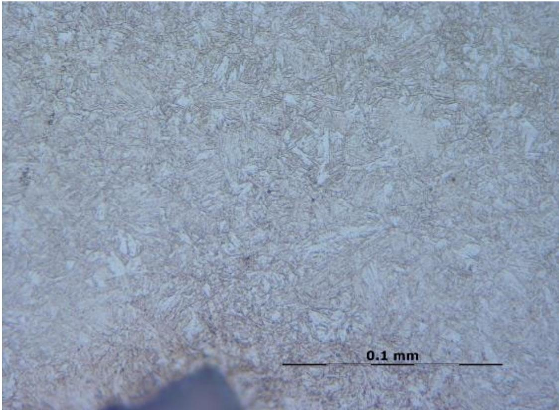
**Figure B-8-7** Cross section, link BJC/5-10: Quenched and tempered microstructure close to outer surface.
