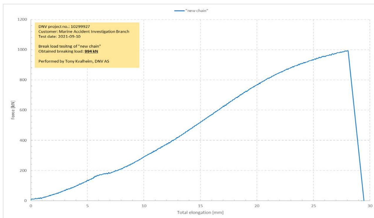
**Figure 4-44 Part BJC/2, unused reference chain, tension versus total elongation.**
