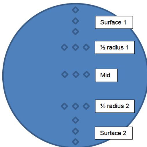
**Figure 4-41 Drawing showing the schematic position of the hardness measurements. Note that the drawing is not to scale. The distance between the measurements in each group is 1 mm.**
