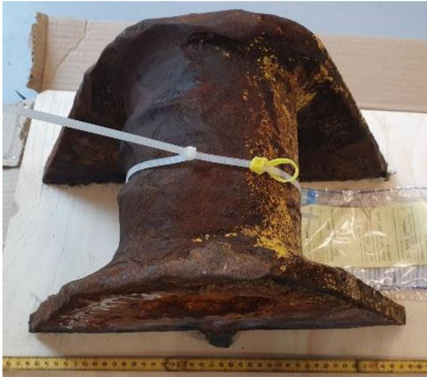
**Figure 4-6** Sample MPH/CM/PORT/3 (PORT/3), portside derrick head.
