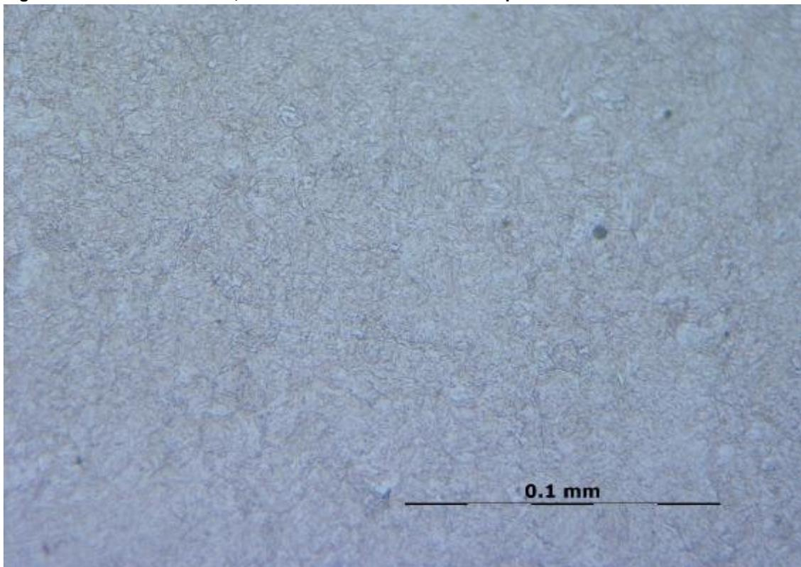
**Figure B-8-2** Cross section, link BJC/1-5: Quenched and tempered microstructure ca 10 mm from outer surface.
