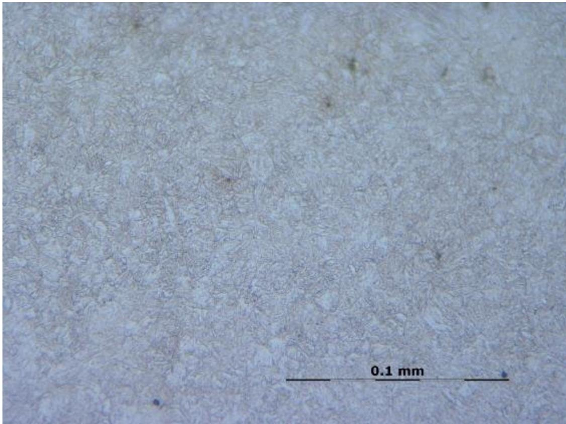
**Figure B-8-8** Cross section, link BJC/5-10: Quenched and tempered microstructure ca 10 mm from outer surface.
