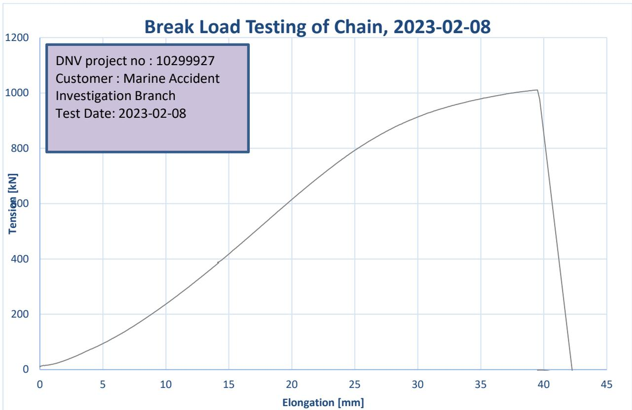
Figure 3-16 Part MJA/4: Tension versus total elongation for break load testing.
