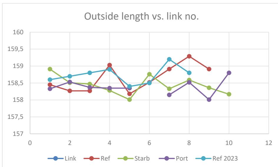
**Figure 3-8** Measured outer length plotted versus link number for all examined chain segments.
