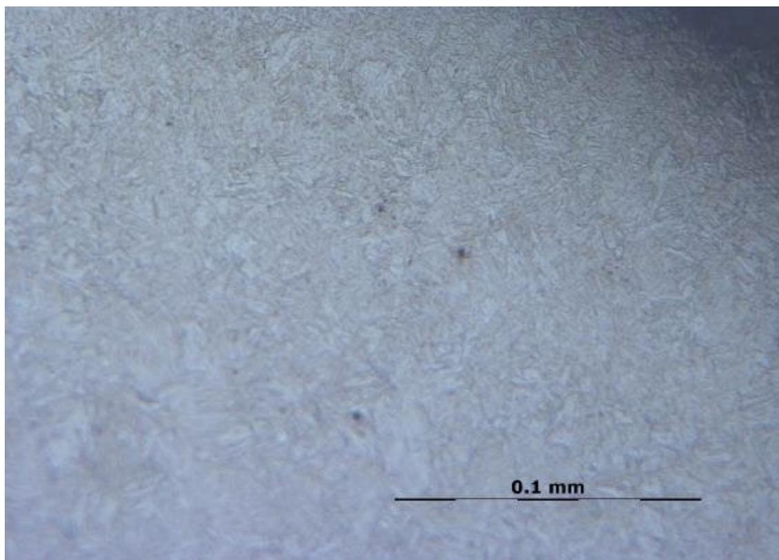
**Figure B-8-5** Cross section, link BJC/3-1: Quenched and tempered microstructure close to outer surface.
