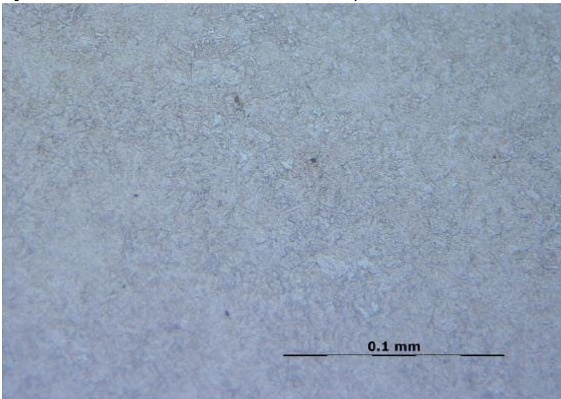
**Figure B-8-4** Cross section, link BJC/2-9: Quenched and tempered microstructure ca 10 mm from outer surface.
