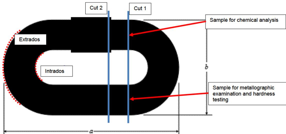
**Figure 4-10** Position of samples for testing. The two blue lines show the cutting positions. All testing (hardness, metallographic examination and chemical analysis) is performed on cut surface 1. The areas denoted extrados and intrados are shown in the drawing.
