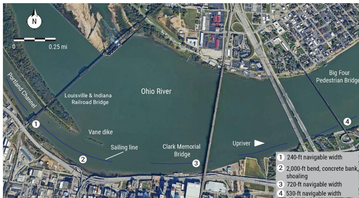
**Figure 7.** Navigational considerations for a vessel transiting upriver on the portion of the Ohio River between the Louisville and Indiana Railroad Bridge and the Big Four Pedestrian Bridge. (Background source: Google Earth)
