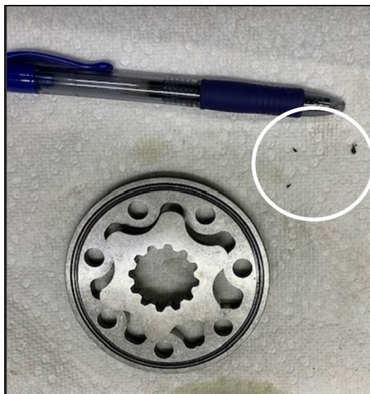
Figure 10. Debris (circled) found in no. 1 steering gear control motor aboard the American Mariner . (Source: Coast Guard)
