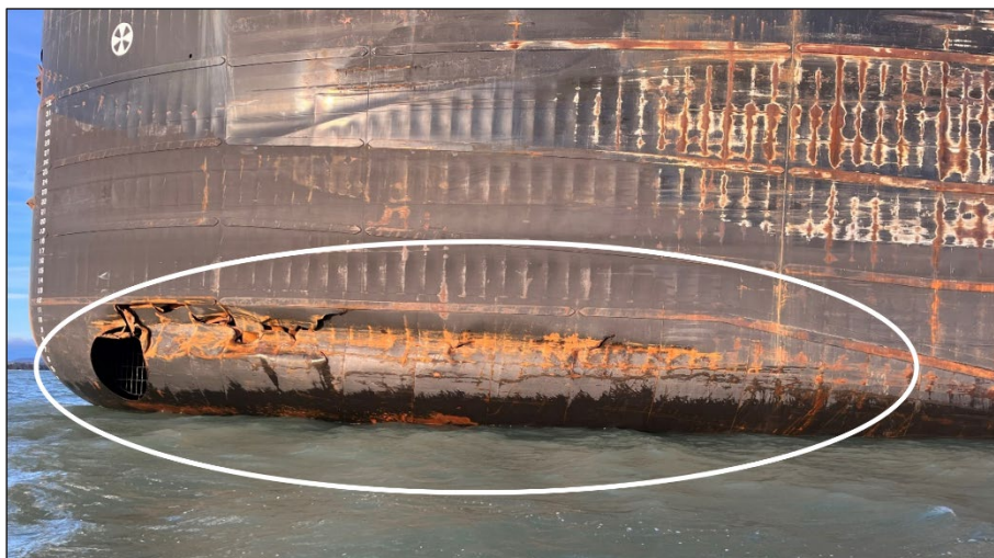
Figure 6. Damage to the port side of the American Mariner (circled) after striking the Munuscong Channel Junction Light. (Source: Coast Guard)
