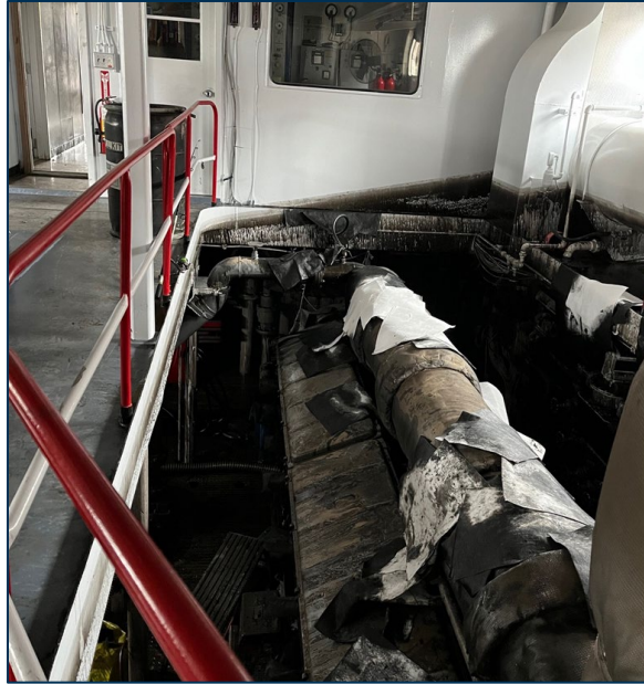
Figure 7. Tom Frazier's engine room, looking forward. The oil-coated bulkheads show the height of water and angle of list before dewatering. (Source: Coast Guard)
