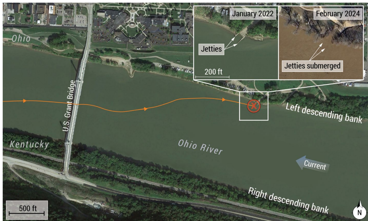
Figure 5. Trackline of Tom Frazier tow as the vessel transited through the U.S. Grant Bridge and toward the right descending bank. Inset satellite photos show the jetties visible on January 26, 2022 (17.4 to 18.5 feet at the Portsmouth gage) and submerged on February 14, 2024 (28.7 to 31.6 feet at the Portsmouth gage). (Background source: Google Earth; trackline source: Tom Frazier automatic identification system; gage data: United States Geological Survey)
