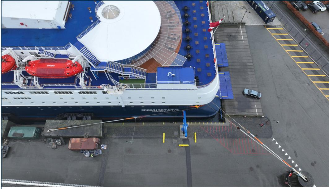
Figure 3: CROWN SEAWAYS' aft mooring configuration in Copenhagen
