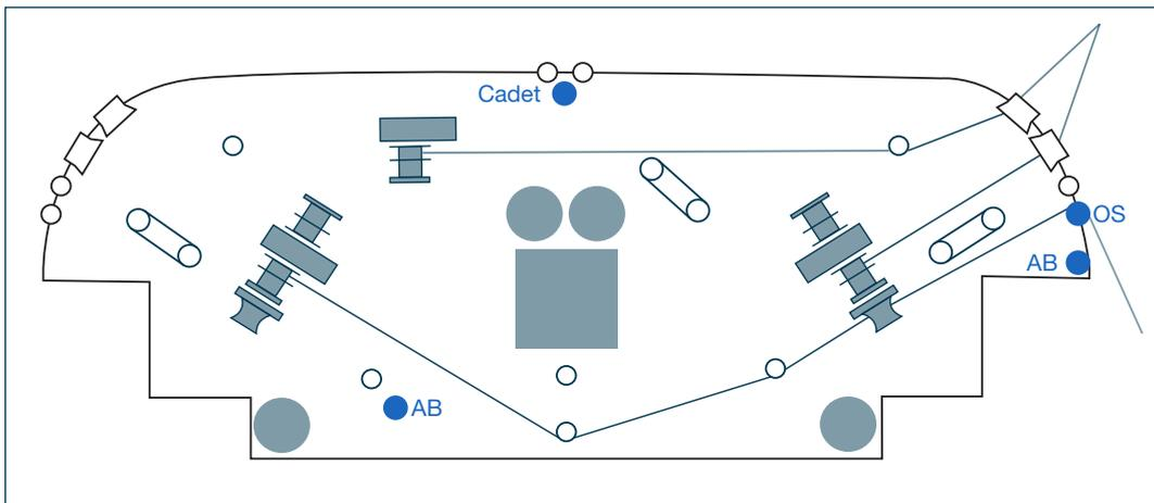
Figure 4: The crew members' positions on the aft mooring station
