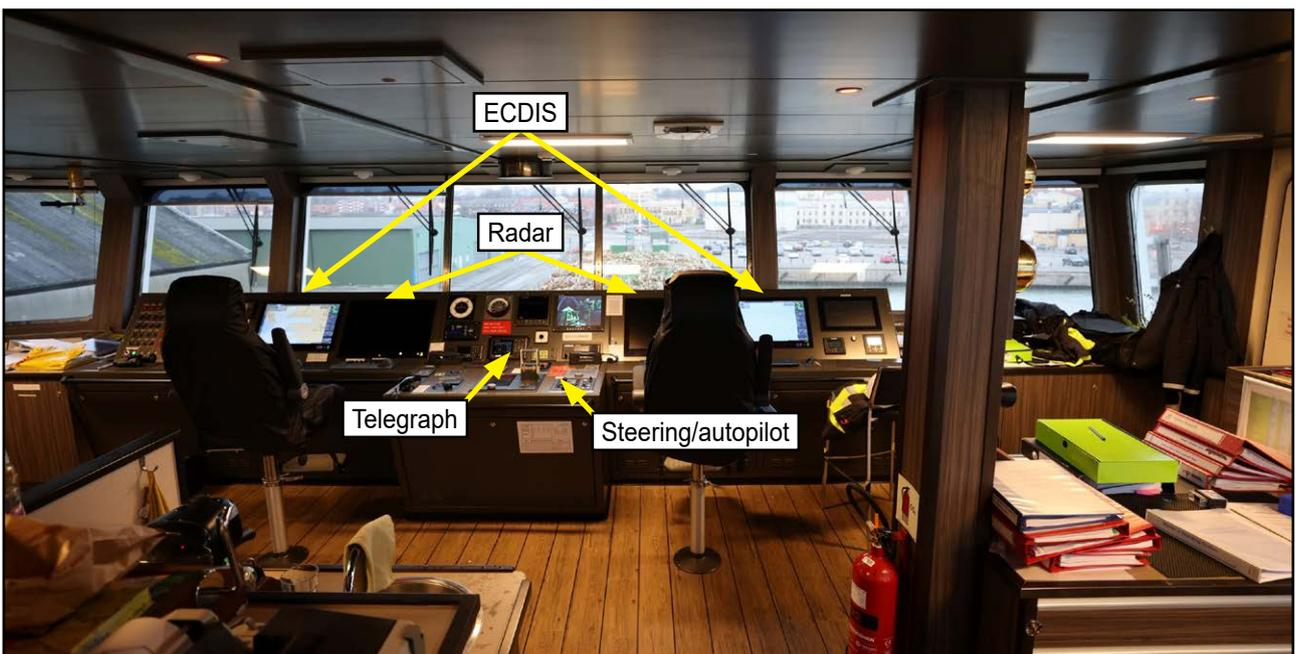
**Figure 3:** *Scot Carrier*'s bridge, showing displays and course and engine controls
