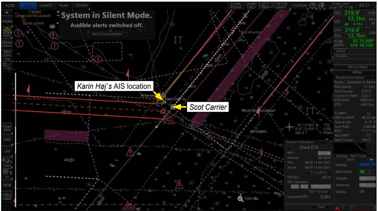
Figure 7: Scot Carrier's starboard ECDIS image at 0321, before altering course
