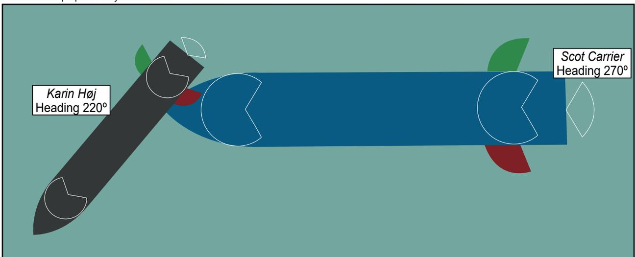
Figure 10: Collision angle (50°)
