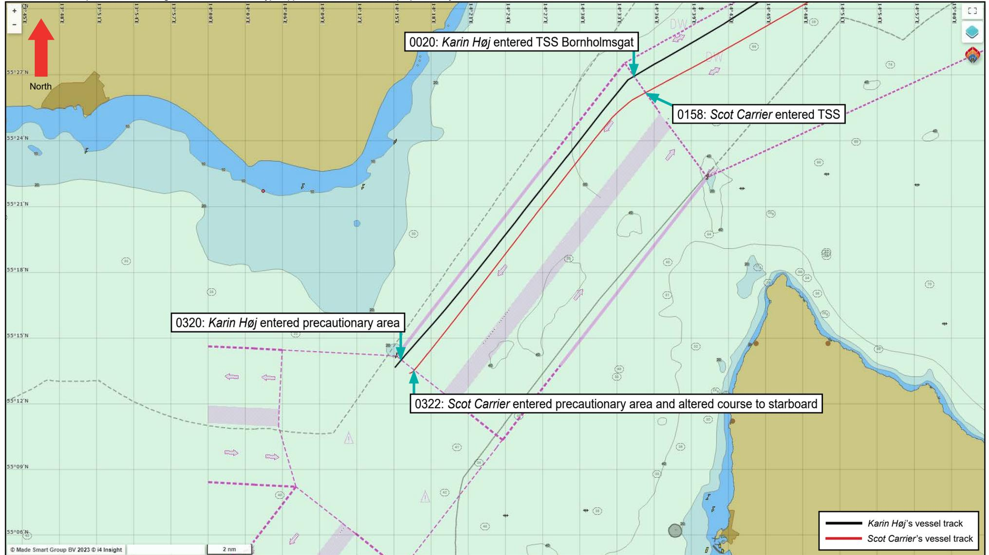
Figure 4: Vessels' routes through Bornholmstrait traffic separation scheme
