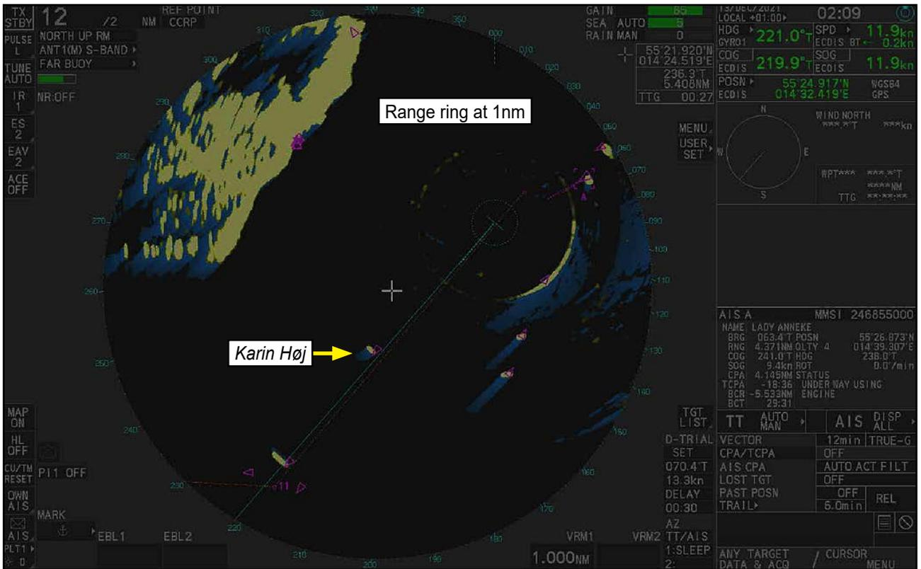
Figure 5: Scot Carrier's starboard radar image showing position of Karin Høj at 0209
