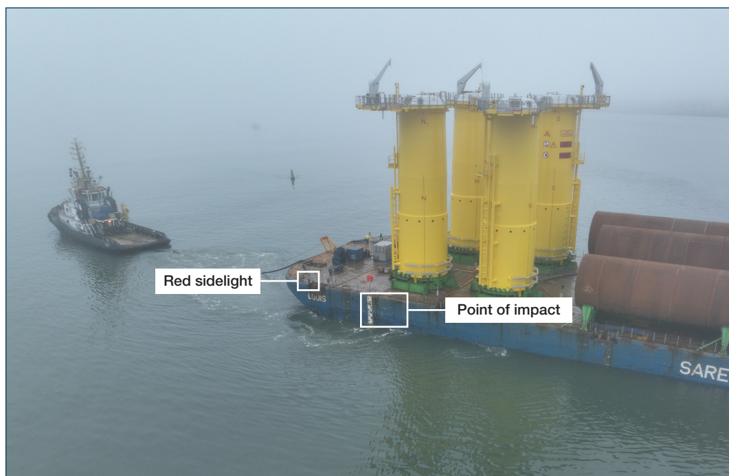
Figure 9: Location of impact on port side of LOUIS' bow. Source: DMAIB
