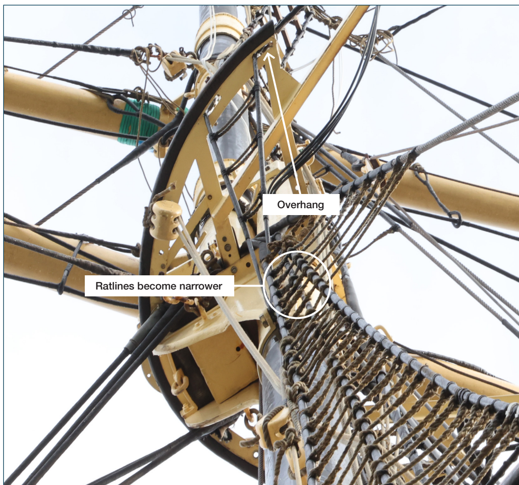
Figure 9: Shroud under topmast crosstrees on the fore-topgallant mast. Source: DMAIB
