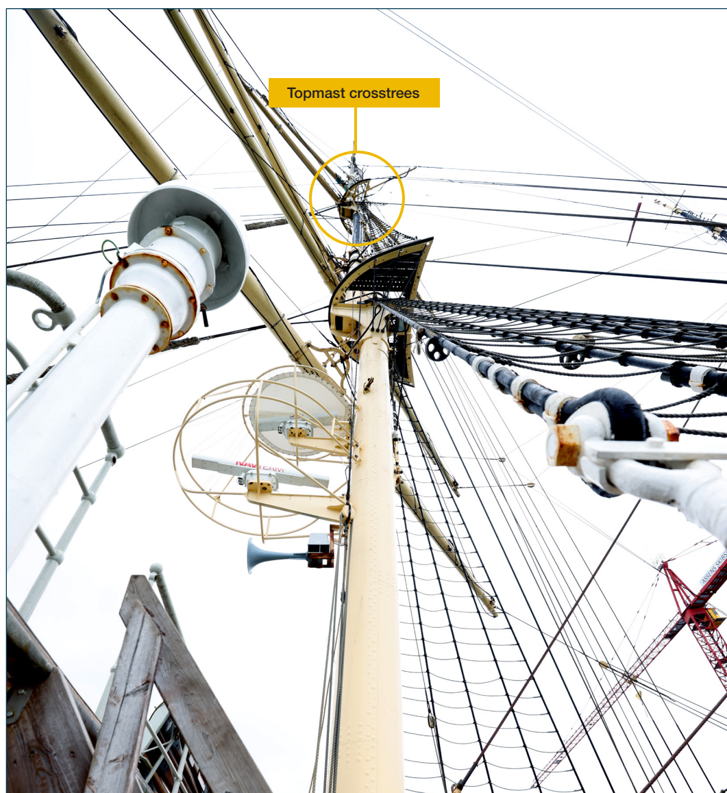
Figure 8: Topmast crosstrees on the fore-topgallant mast seen from the pin rack Source: DMAIB
