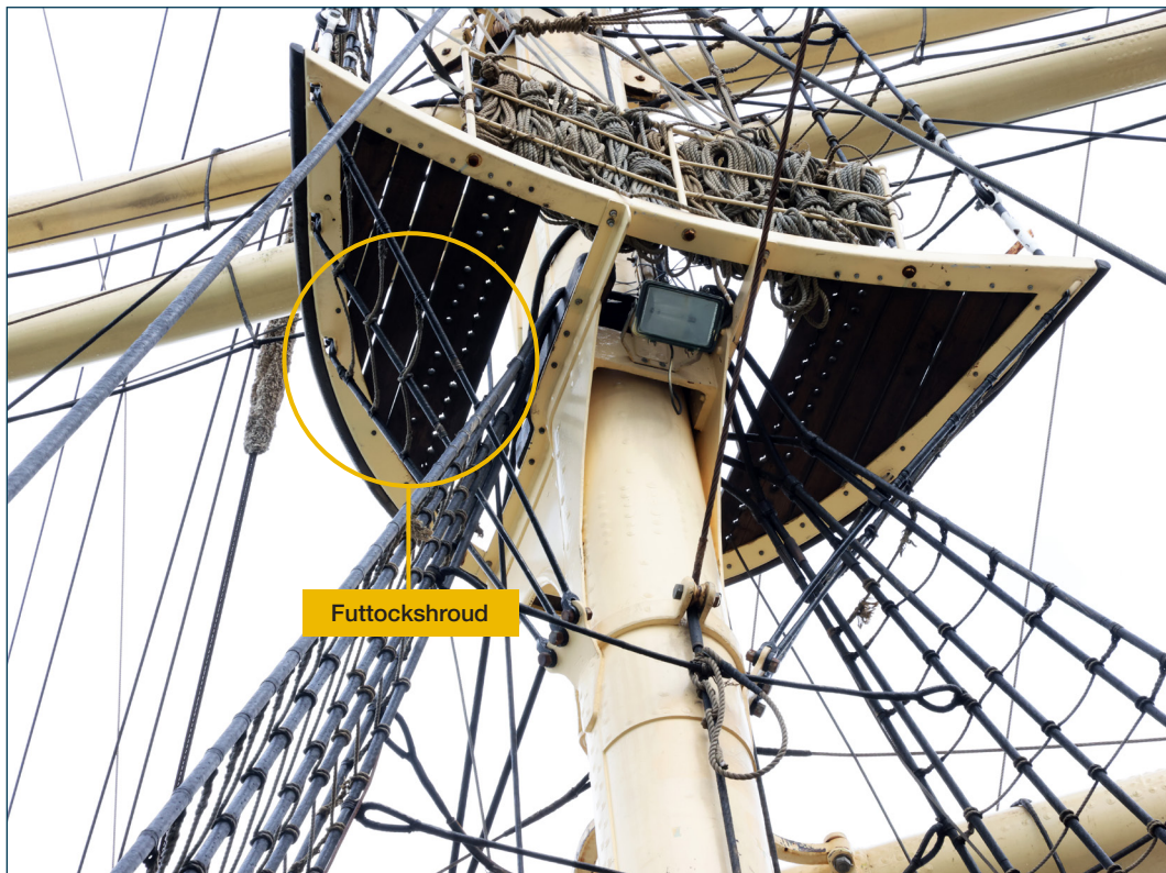
Figure 5: The underside of the top in the fore-topgallant mast. Source: DMAIB
