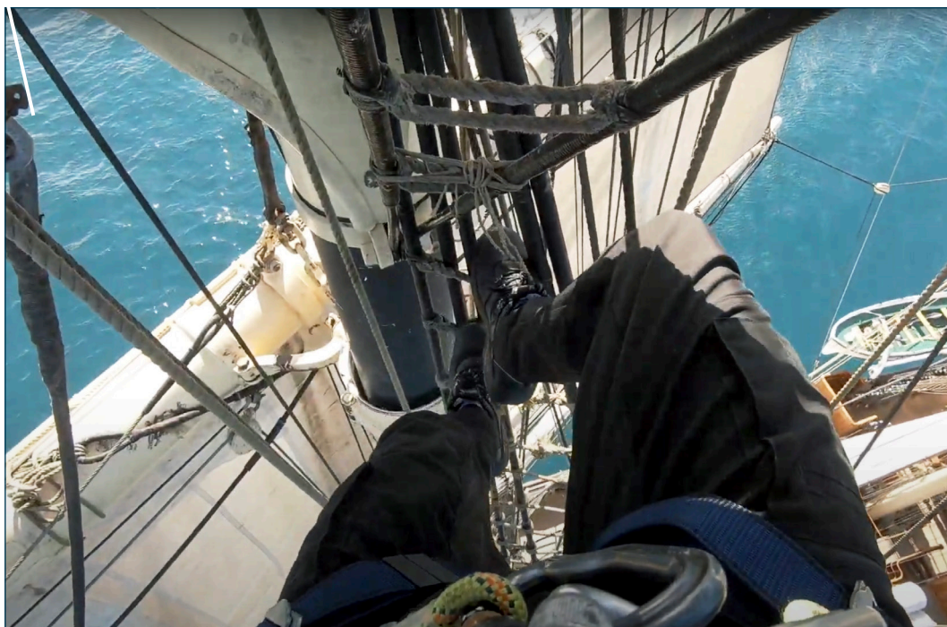
Figure 10: Feet in ratlines under the topmast crosstrees (in the mainmast). Source: Kasper Feder, YouTube (dk), 2021
