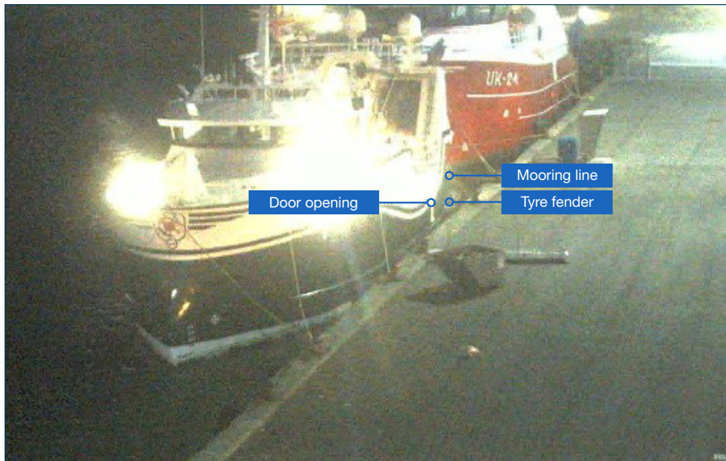
Figure 4: Deckhand grabs on to mooring line, step on the tyre fender and leans upper-body into door opening. Source: DMAIB
