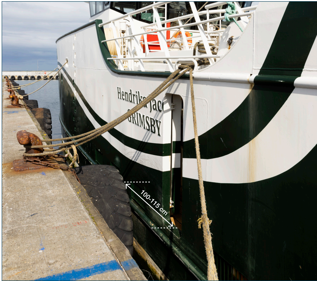
Figure 14: Actual distance to straddle when stepping from tyre fender to door opening. 30 May 2022 at 1730. Source: DMAIB.
