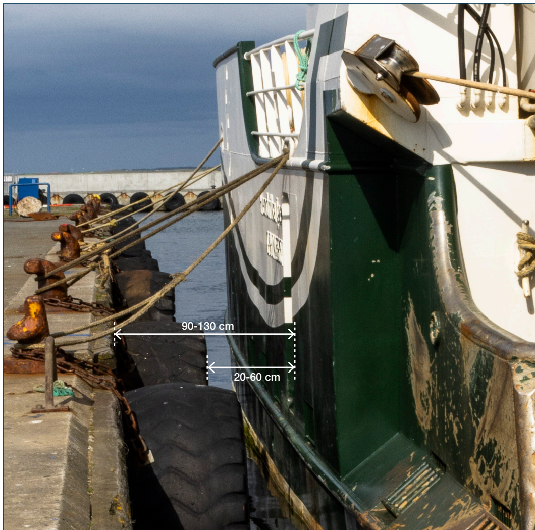
Figure 11: Distance between quay and ship. Source: DMAIB
