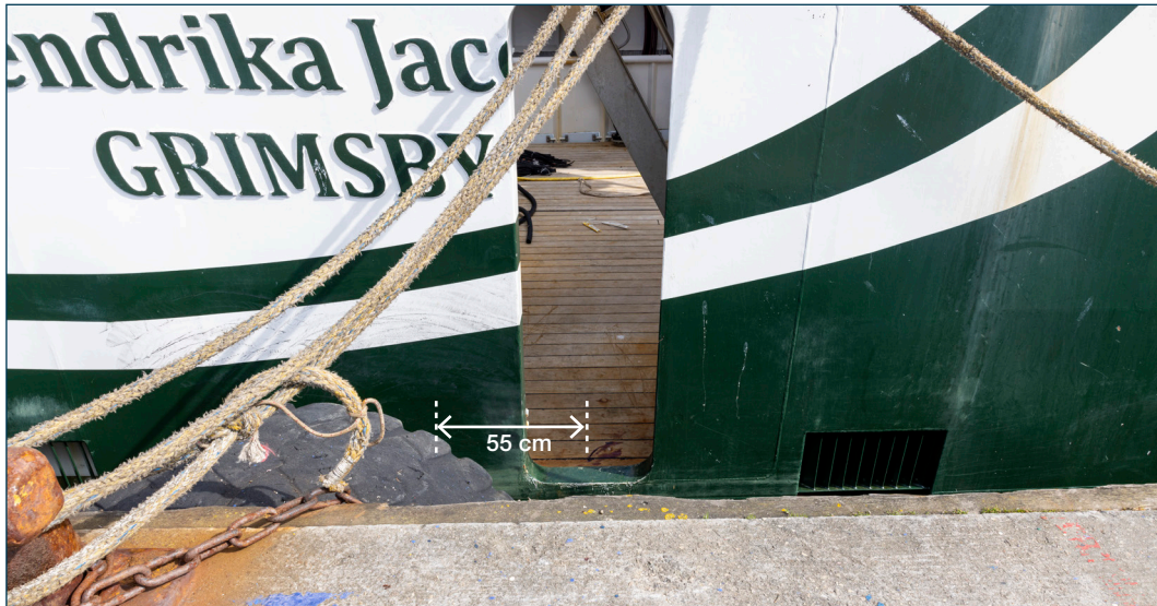
Figure 12: Horizontal offset between stepping point on tyre fender and door opening. 30 May 2022 at 1730. Source: DMAIB
